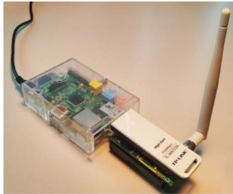
Figure 3.22 Picture of the integrated node. A Raspberry Pi hosts a TelosB mote as IEEE 802.15.4 interface and a TP-LINK as IEEE 802.11s interface.
