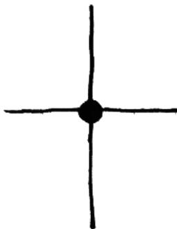
**Figure D-3.** *Schematic symbol showing connected wires*
