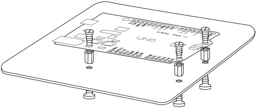
**Figure 8-32.** *Arduino mounted on standoffs inside case*
