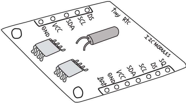
**Figure 8-2.** *TinyRTC Real Time Clock module*
