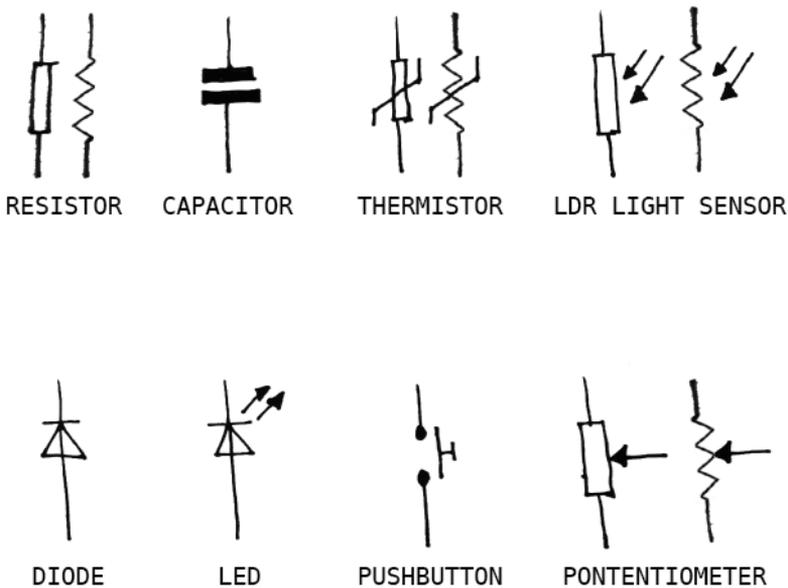
**Figure D-4.** *Common schematic symbols seen in Arduino circuits*
