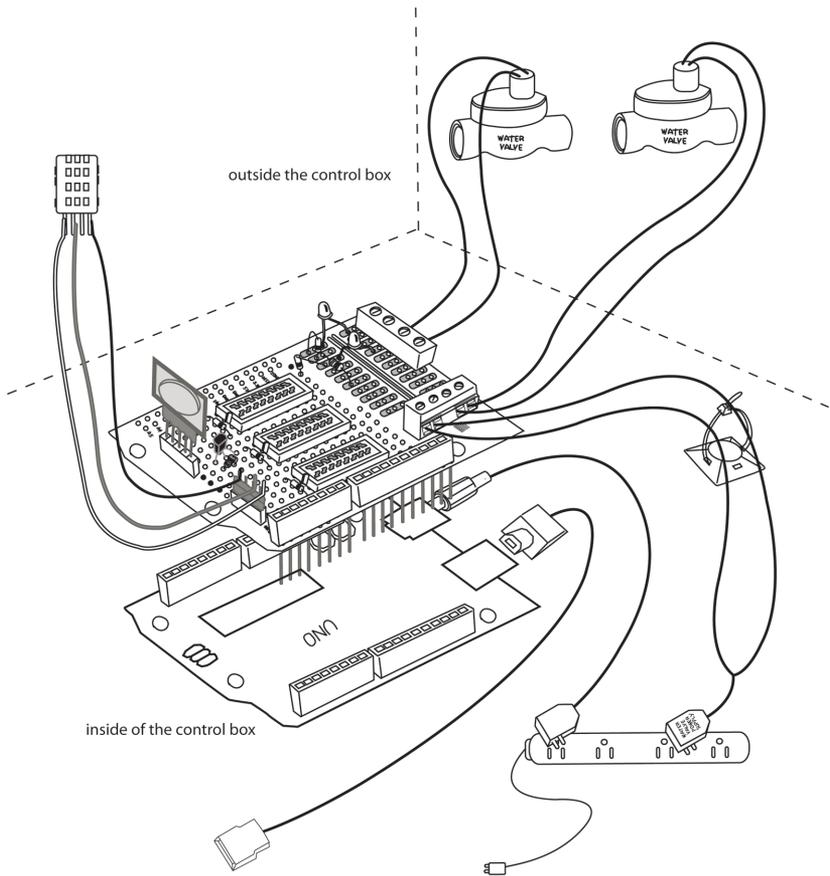
**Figure 8-34.** Completed automatic garden-irrigation system
