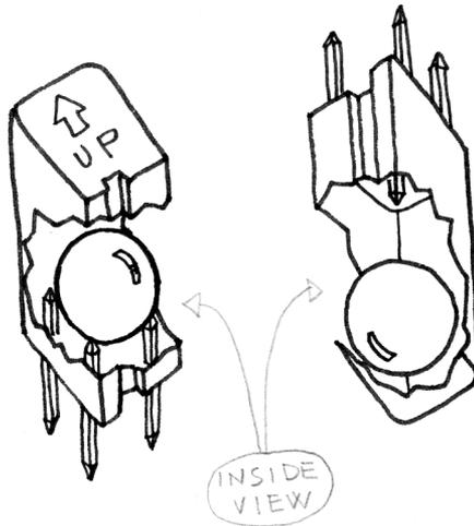
**Figure 5-1.** *The inside of a tilt sensor*
