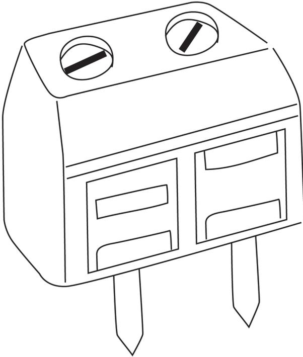
**Figure 8-8.** *Good-quality screw terminal with two positions*
