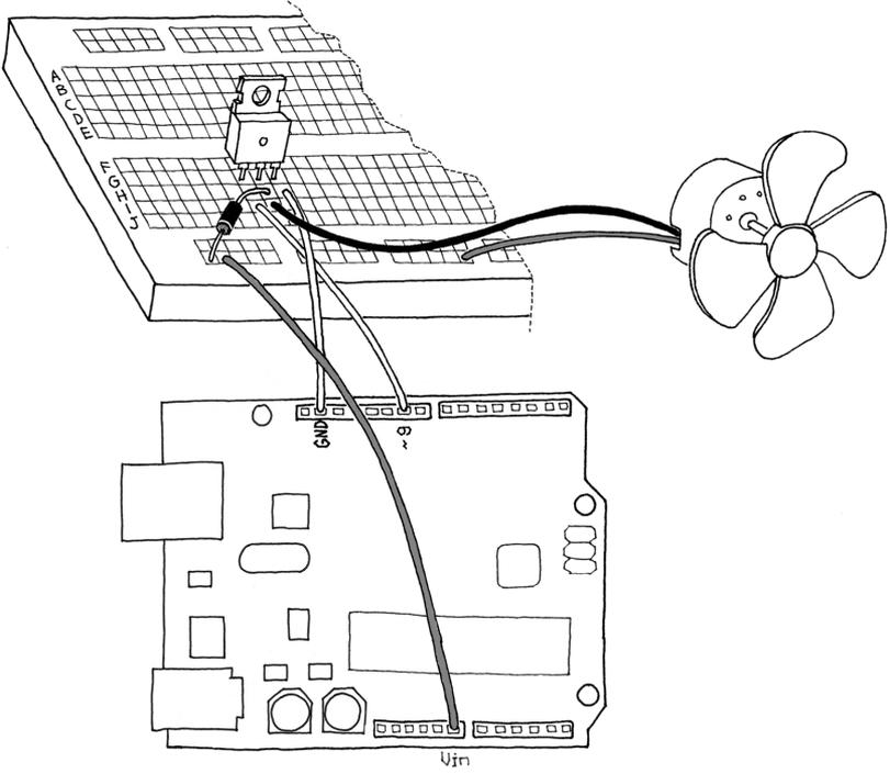
**Figure 5-7.** A motor circuit for Arduino
