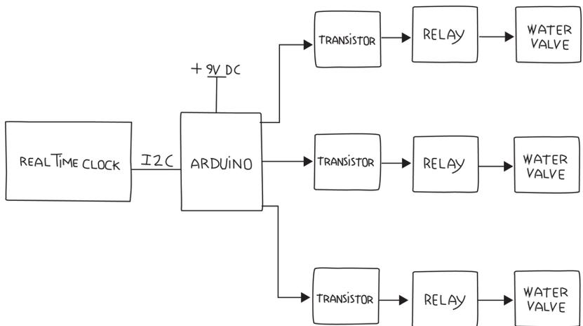
**Figure 8-1.** Block diagram showing Real Time Clock, Arduino, MOSFETs, relays, valves, and power supplies
