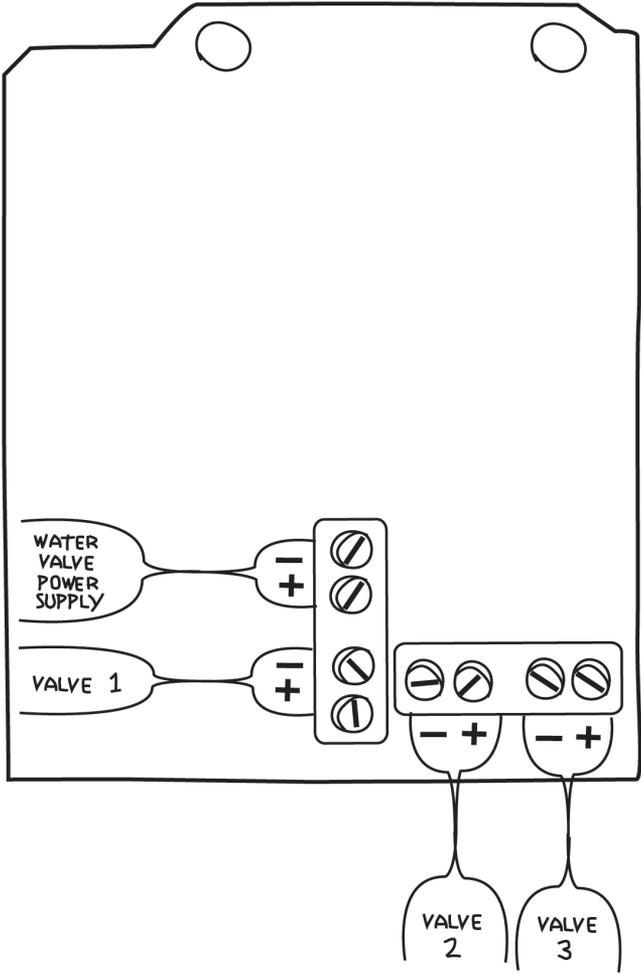
**Figure 8-21.** Documenting which screw terminal does what
