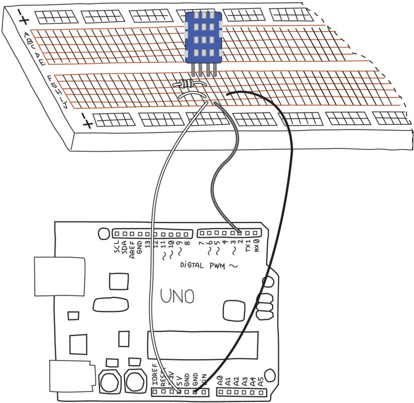
**Figure 8-14.** Pictorial circuit diagram for testing the DHT11 Temperature and Humidity Sensor
