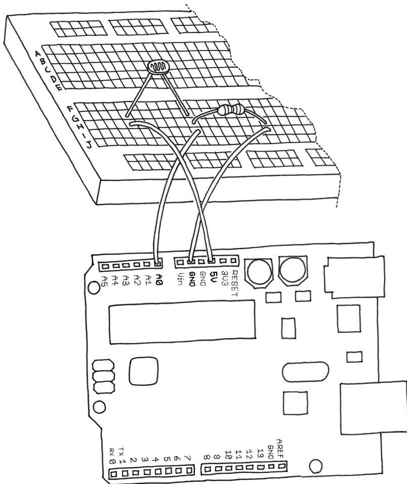
**Figure 5-6.** An analogue sensor circuit
