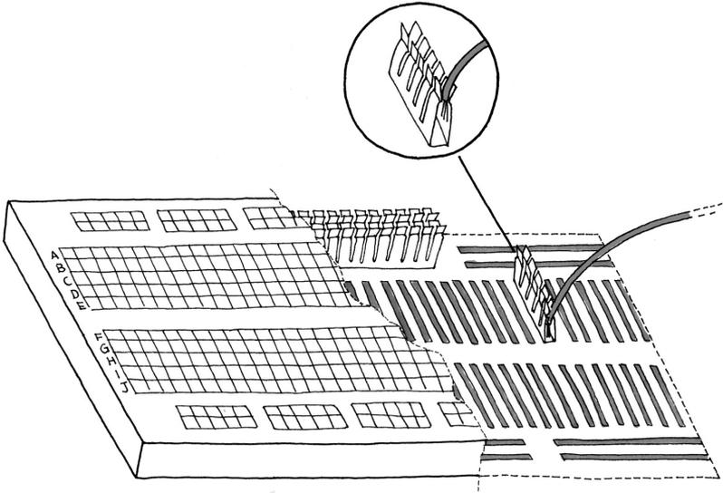
**Figure A-1.** *The solderless breadboard*
