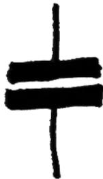
**Figure D-1.** Schematic symbol for a capacitor
