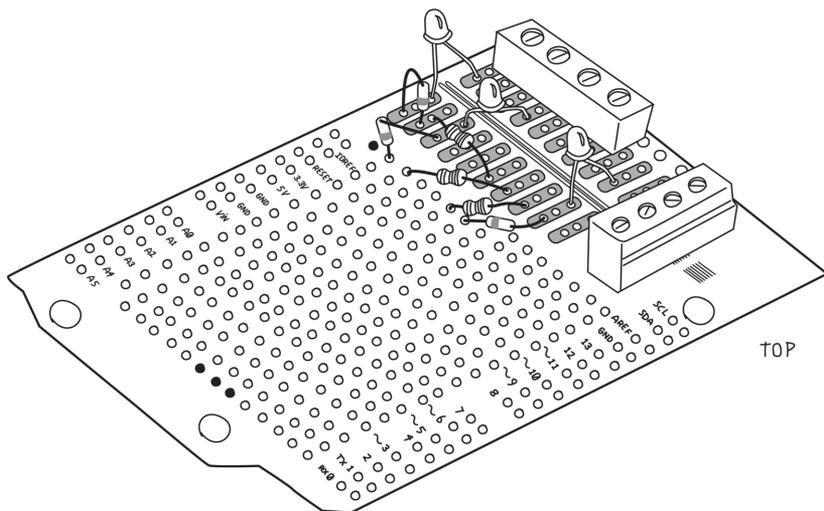
**Figure 8-22.** Top view showing LED, resistor, and diode placement
